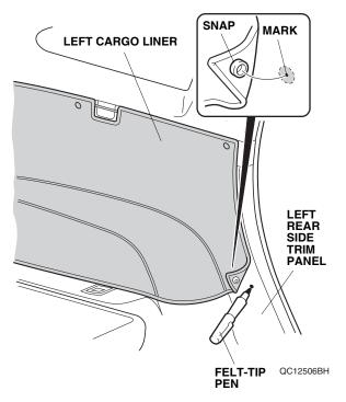
13. Fold the cargo liner. Using a pushpin, pierce the mark on the left rear side trim panel.
