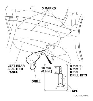
7. Press one well nut into the each hole in the left rear side trim panel.
