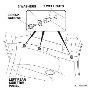
8. Place a washer onto the snap-screw and install three snap-screws into the each well nut. Securely tighten the snap-screws.
