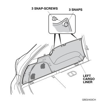
12. Fit the corners of the left cargo liner around the left rear side trim panel. Adjust the left cargo liner so that it fits smoothly over the edges. Using a felt-tip pen, mark the snap location of the left cargo liner on the left rear side trim panel.
