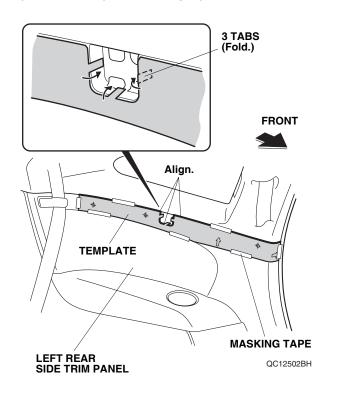
4. Using a pushpin, pierce the left rear side trim panel through the template at the three locations shown on the template.
