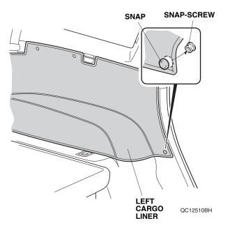
Turn the template over, and repeat steps 3 through 17 to install the right cargo liner on the right side of the vehicle.
